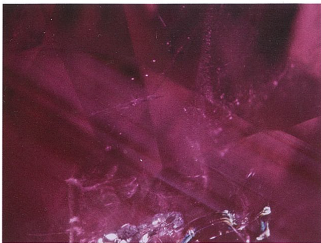
Figure 14: Common inclusion features in the rubies from Tajikistan consist of very fine-grained planar clouds that can have a whitish or faint bluish appearance when viewed with fibre-optic lighting. Photomicrograph by C. P. Smith; magnified 30 \times .
