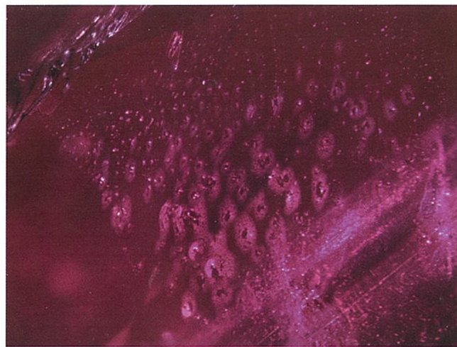
Figure 15: The most recognisable and diagnostic inclusion feature for rubies of Tajik origin consists of small negative crystals, each individually associated with basal-oriented thin films. These occur in groups along planar concentrations, as shown here, or as isolated features. Also present are fine, reflective stringers. Photomicrograph by C. P. Smith; magnified 38 \times .
